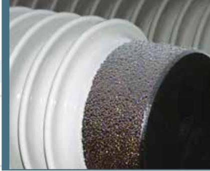
Sand bands bonded to the porcelain by glaze provide a rough surface for permanently attaching the hardware and distributing loading evenly through the porcelain. The high strength compression sand is manufactured by **PPC** Insulators to match the characteristics of the porcelain body.
