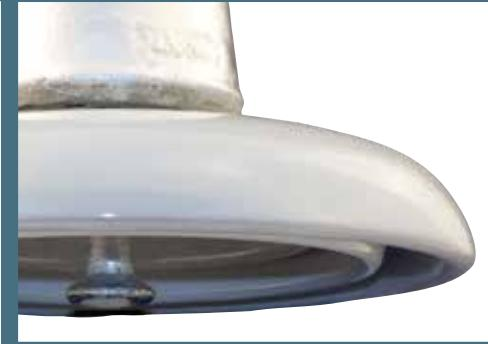
The umbrella type spreading porcelain shell or shed protects the leakage corrugations on the underside of the insulator from contamination and mechanical damage. The sheds are designed to provide optimum normal and protected leakage distance in relation to size and shape.
