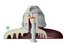
**A** = Puncture distance **B** = Flashover distance **C** = Most common puncture
