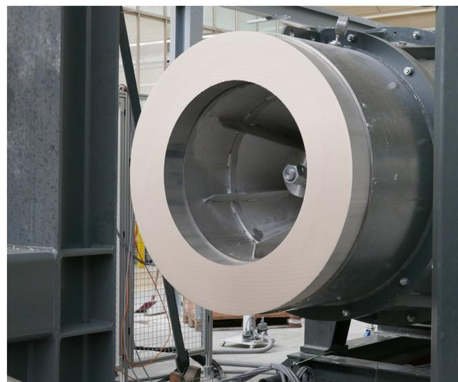
With the new XXL Extruder, PPC Insulators is capable of producing multipart insulators up to 1,100 mm in diameter and exceeding 11,000 mm in length and single piece hollow insulators with 2,750 mm length, ranging from 72 kV up to 1,200 kV AC and 1,100 kV DC,
