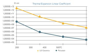
High resistivity at elevated temperatures whereby electrical breakdown caused by high leakage current through the material is avoided.
