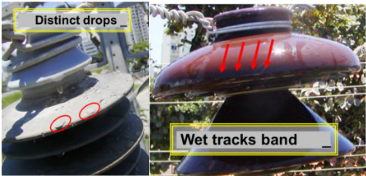
Fig. 6 – Hydrophobicity and the wet band area
