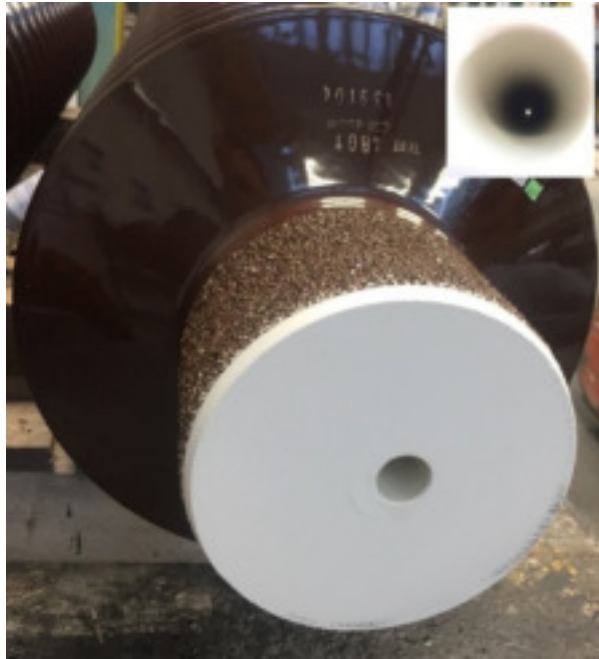
Fig 3: Fiber Optic Hole Post Insulator after firing and cutting.
