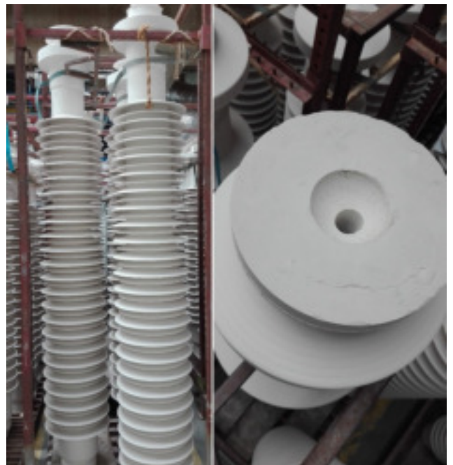
Fig 2. Fiber Optic Hole Post insulator ready for glazing and firing.
