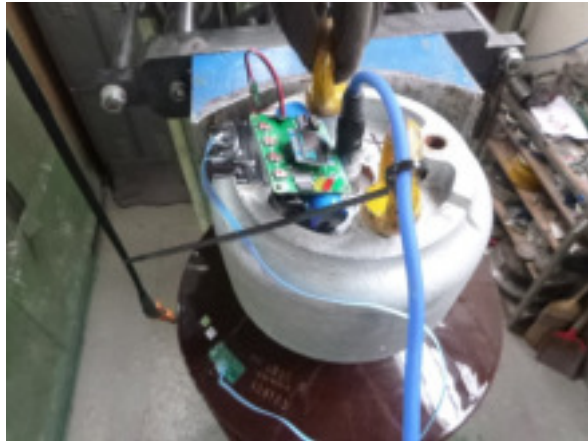
Fig 7: Test Set up with a microphone inside the Fiber Optic Hole and Accelerometer glued on the shed.
