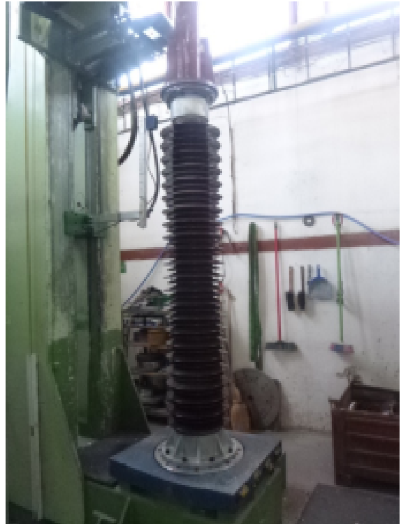
Fig 5: Bending test at PPC Insulators CAB.
