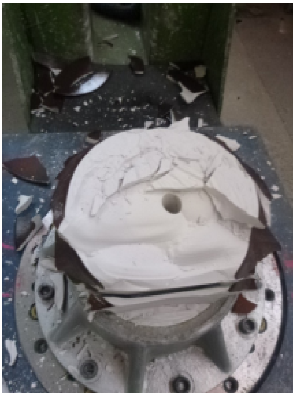
Fig 6: The broken Fiber Optic Post Insulator. The Fiber Optic Hole is not affecting the breakage mechanism.
