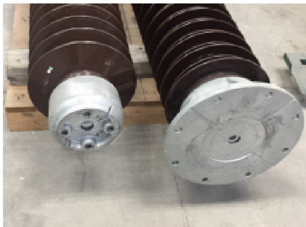
Fig 4: Assembled C30-850 Fiber Optic Post Insulator ready for testing.
