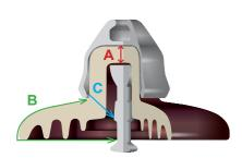
**A** = Puncture distance **B** = Flashover distance **C** = Most common puncture
