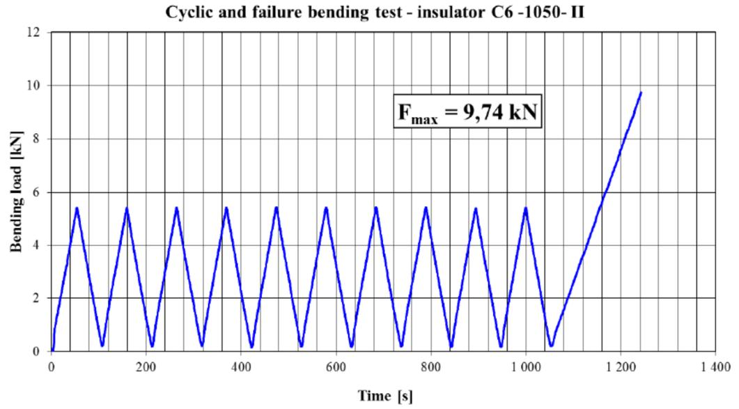
Graph. 3. Cyclic and Bending Failure Test with Isostatic insulators.
