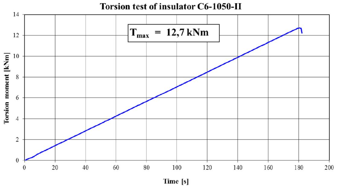
Graph. 6. Torsion Test with Plastic Insulator
