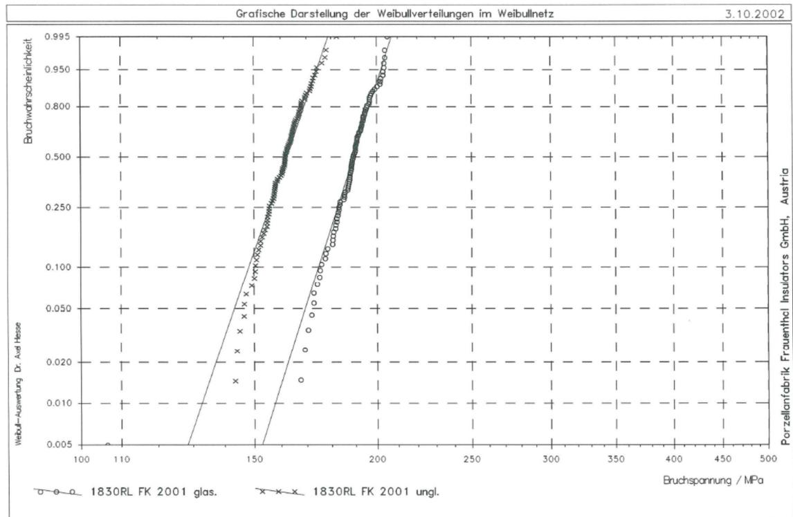
Graph. 2: 3-Point-Bending Test Weibull-Analyse of Plastic C 130 Porcelain
