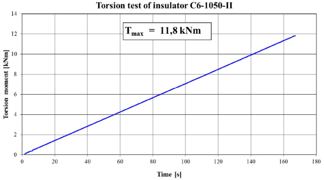
Graph. 5. Torsion Test with Isostatic Insulators.
