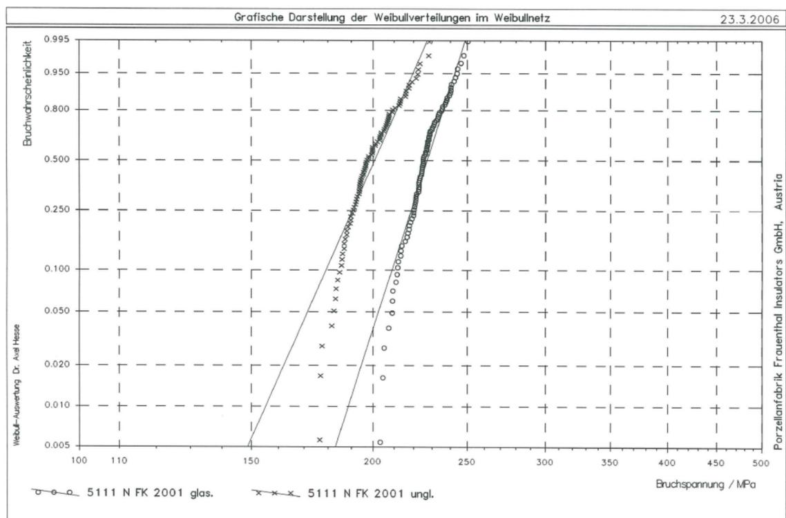
Graph. 1: 3-Point-Bending Test Weibull-Analysis of Isostatic C 130 Porcelain
