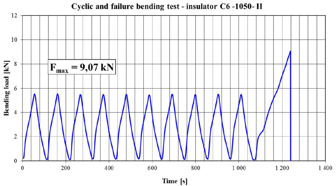
Graph. 4. Cyclic and Bending Failure Test with Plastic Insulators.
