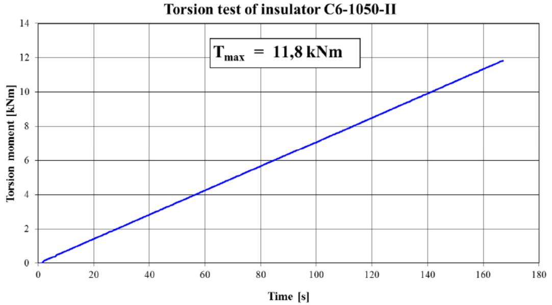
Graph. 5. Torsion Test with Isostatic Insulators.
