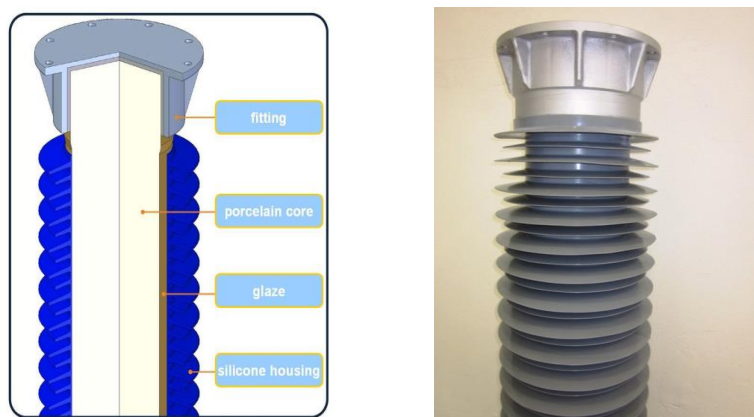
Fig. II: Hybrid solid core post insulator
