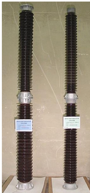
Photo 3: Post C9-1800 with traditional- and InsuLite design
