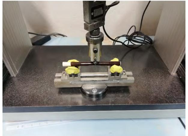
Fig 6. 3-point bending machine.
