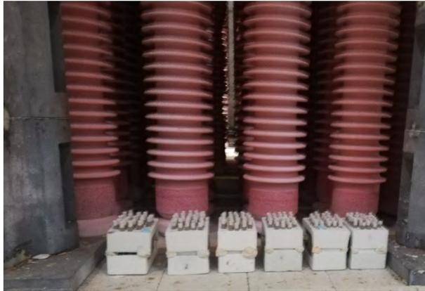
Fig 4. Samples ready on kiln for firing.
