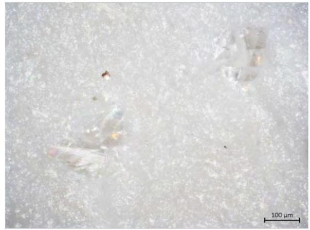
Fig 11: two 200 μm quartz crystals on
