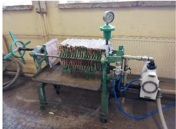
Fig 1. The laboratory filter-press
