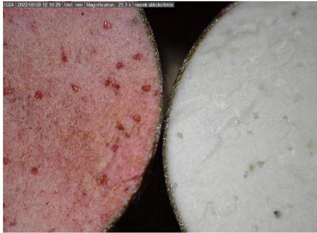
Fig.13: Breakage surface after 30'000 cycles. The dye penetration test reveals the quartz particles clearly as the liquid penetrates the microcracks of the crystal. Anyhow there is no visible crack propagation on the base material.
