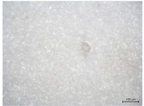
A dye penetration test was executed to reveal the potential cracks on the breakage surface.
