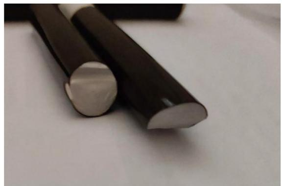
Fig 8. Broken test bar at 3-point bending test.
