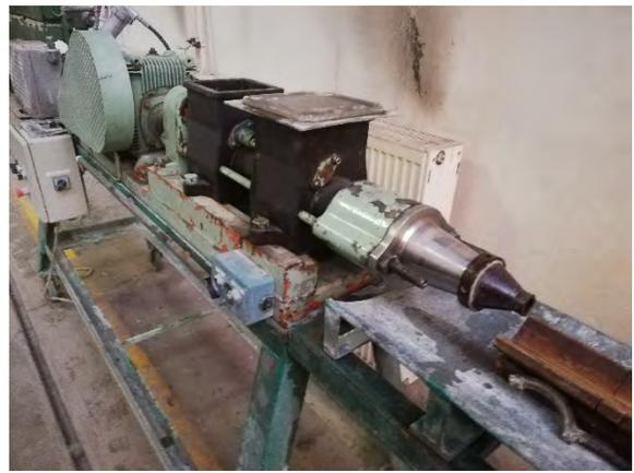
Fig 2. The laboratory extruder.
